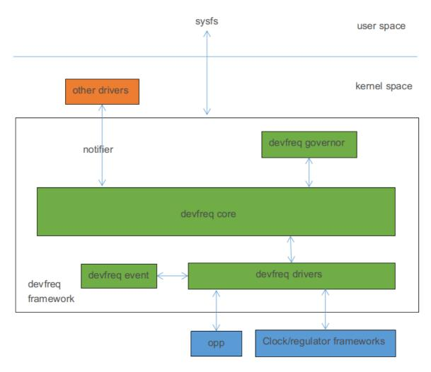
Devfreq governor: It is used to determine when to change the frequency and which frequency will be change to. The kernel includes the following governor:
